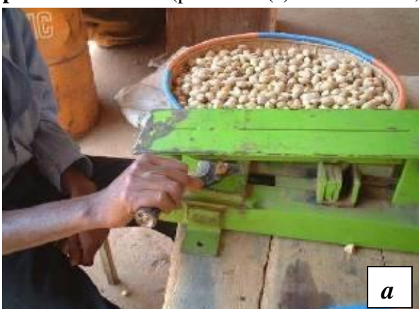
Plate 4: Extraction of Melia seeds from nuts using: (a) Melia nut-cracker and (b) wood plank and knife (photos of (a) KEFRI/JICA, (b) CADEP-SFM/JICA)
